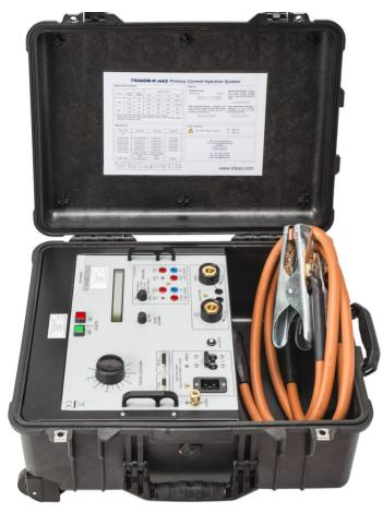
T&R Test Equipment is a market leader in the field of current injection equipment. The range includes secondary injection units with 100A output capability up to 6000A primary injection systems. All have true RMS metering, a flexible timing system, and an easy to understand user interface.
