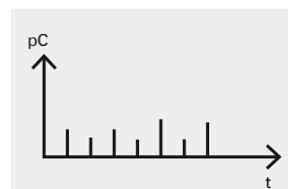
Partial discharge DC
