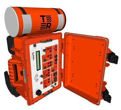
The 50ADM-P is a smaller version of our current injection system the 200ADM-P. The unit has a range of outputs allowing injection of currents between 1mA and 50A. Voltages up to 18V are available on the main outputs. True RMS metering with single cycle capture is provided.
