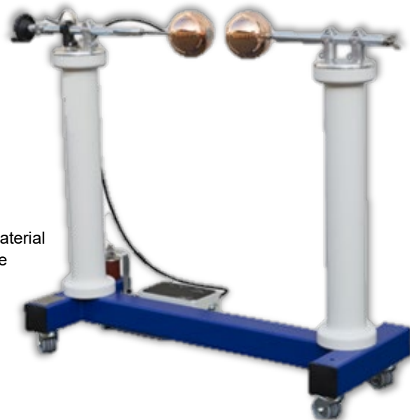
Horizontal Sphere Gap KFS H
